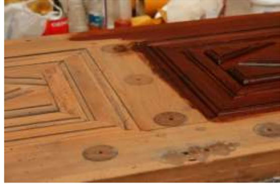
Figure 8: Applying shellac polish (Güneş, 2011).
