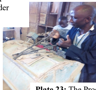
Plate 23: The Process of turning of broken pieces ceramic into ball milling machine so as to grind the waste into finer particles
